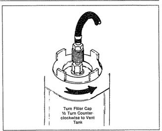
4. Turn gas tank filler cap one-half turn counterclockwise to vent tank.
